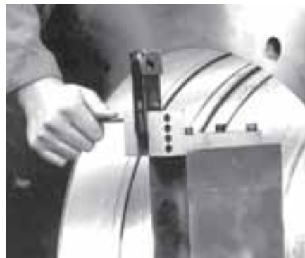
Tool head accepts either HSS tool bits or carbide insert holders as shown here.
