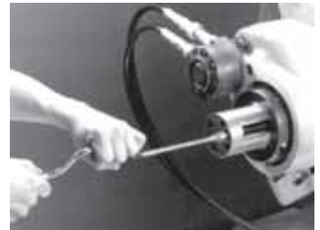
Speed wrench or portable drill motor can be used to move tool head from either end of the bar, with or without the axial feed unit attached.
