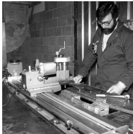
A PM3000 milling a turbine diaphragm at Philadelphia Electric.
